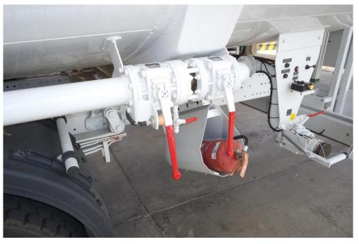
Fueller for defuel service - Where the defuel circuit includes a double valve arrangement (vehicle designs pre-2014), the section of pipe between the valves shall have a low point drain and this shall be checked daily for leakage and flushed each 6 months.
